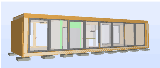
Figure 8. BIM model of the Rooftop building, reduced to the relevant building elements for building energy simulation.
