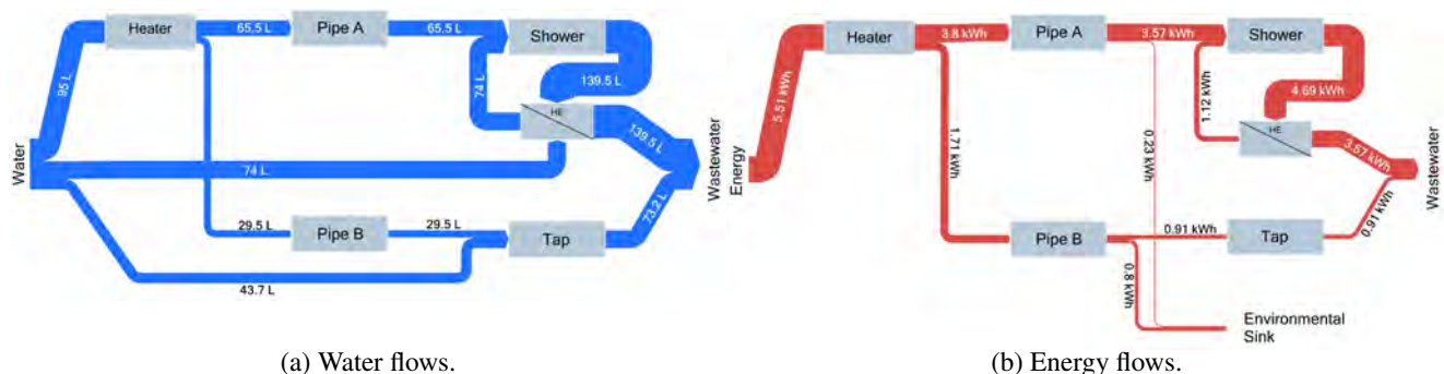
Figure 1. Average daily water and energy flows in a didactical DHW system containing a shower-level heat recovery device (HE).
