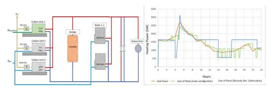
This paper shows and describes a new approach as to how Modelica models can be used to evaluate the dynamic behavior of district heating grids. It furthermore introduces a consistent framework to parameterize these models with GIS-data via the COM interface. The advantages of the shown approach compared to previously used static methods are shown with specific case studies.
