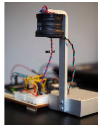
(b) Arduino controlled electromagnetic levitation system.
