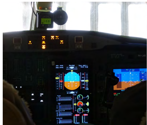
Figure 2. Cockpit instruments in use for flight testing on a Cessna Citation aircraft.
