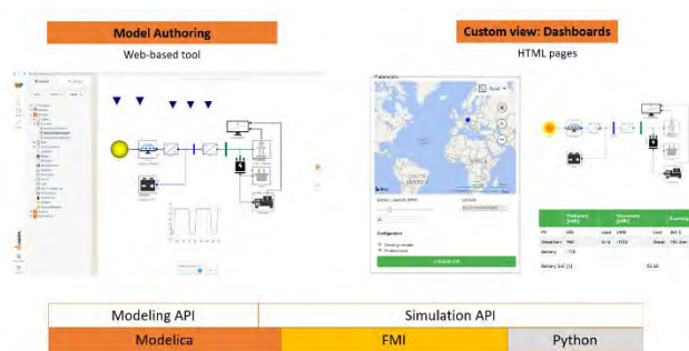
Figure 1 Microgrid models in an architecture overview of Modelon's web-based modeling and simulation platform.
